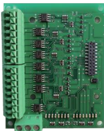
· 02-16swRX 16接点用快速端子板* (16路开关/环回/8路应答, 双向兼容)
